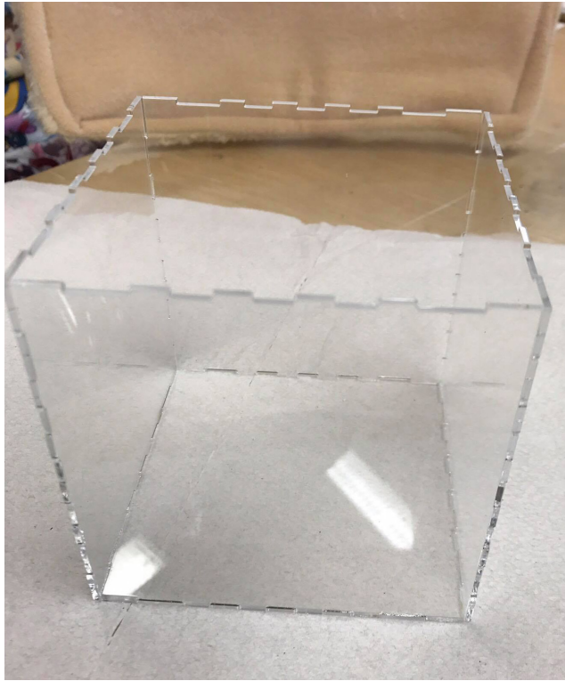
Plexiglass was laser cut then assembled together to form a cube.
